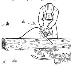
Figure 13 - Bucking Log With Entire Length On Ground
